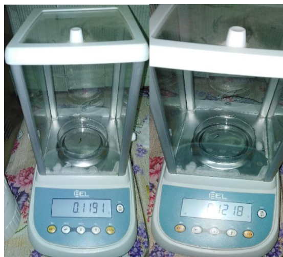
Figure 2: Bel model M214a balance for accurate weighing of mini-implants before and after coating.
