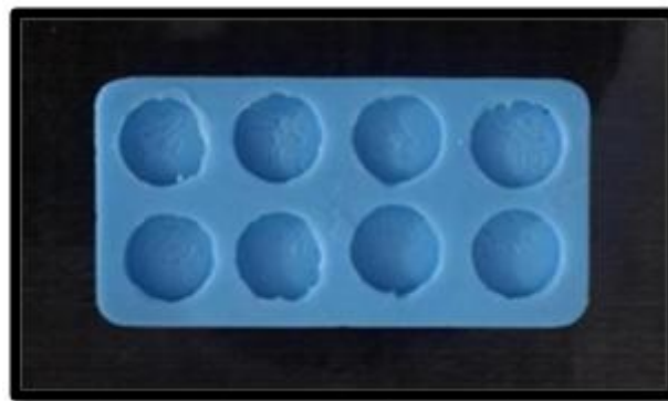
Fig 3: Silicone Jig for Uniform Layering of 1mm
