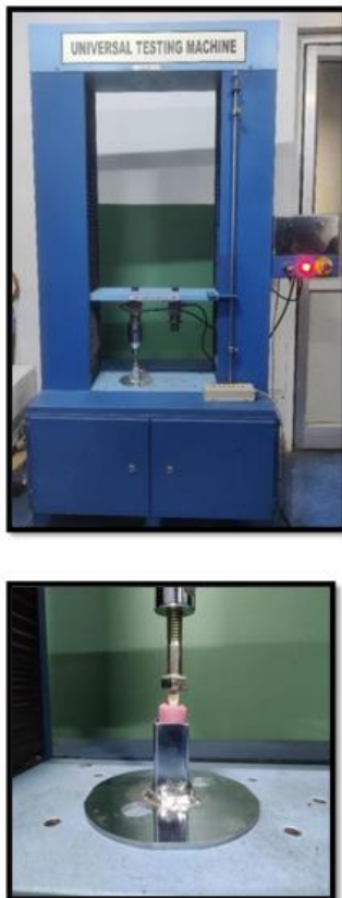
Fig .10: Evaluating fracture resistance under Universal testing machine
