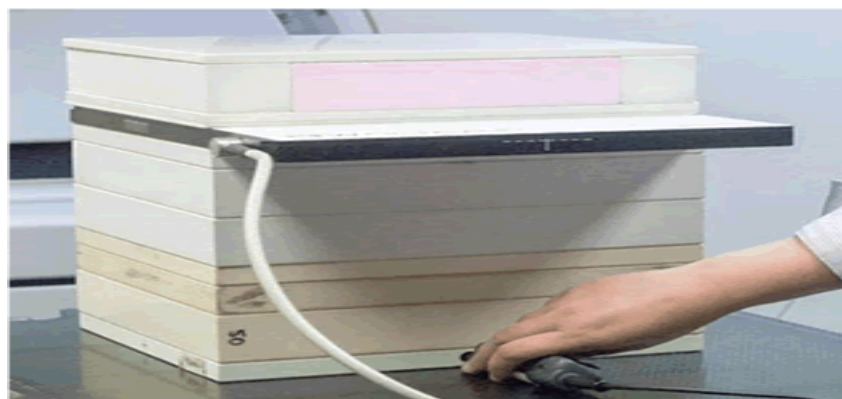
Figure 3: shows the initial evaluation setup utilizing an ionization chamber
