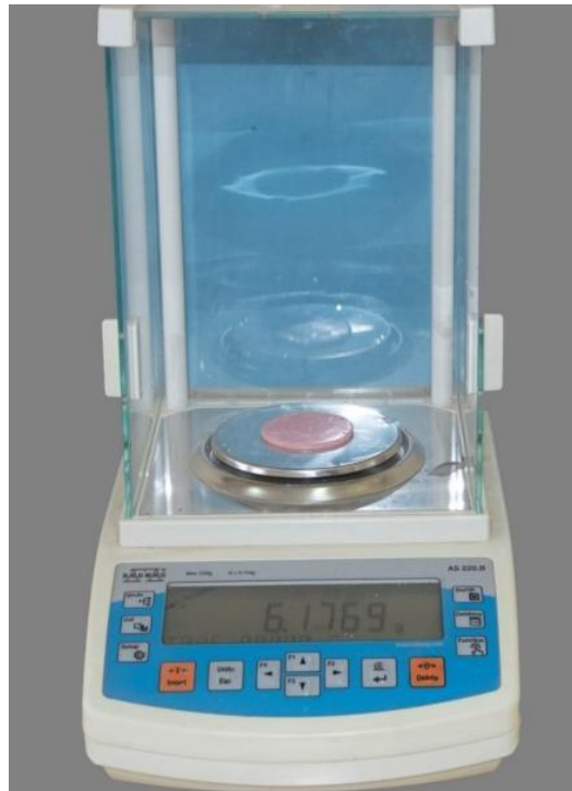
Figure 6: Specimen weighed in electrical balance.
